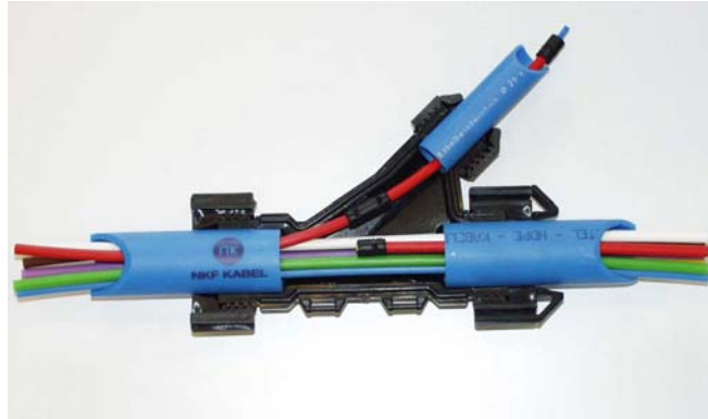
Figure 2 Clip-on separable Y-connector for branching any time and any place, without splicing
