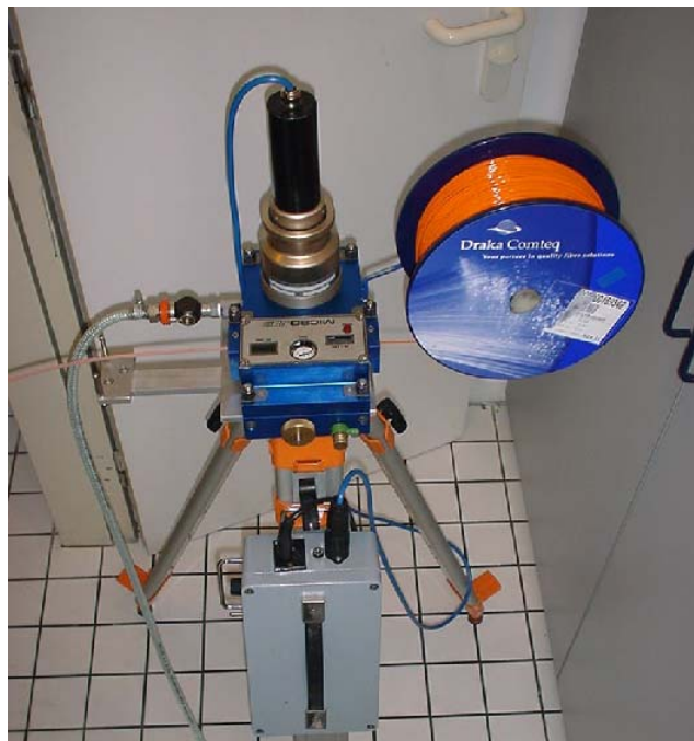
Figure 6 Jetting FttH \mu duct cable
